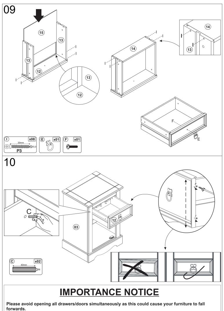
Make sure to secure this piece of furniture to the wall by using fittings below supplied for this purpose.
