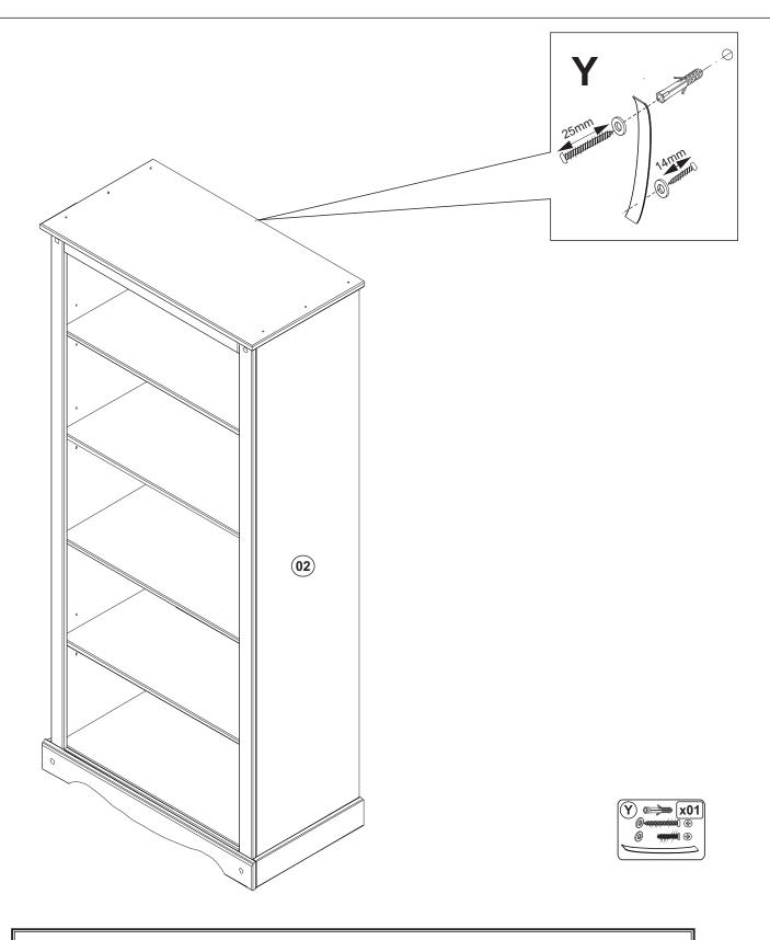
WARNING: CHECK FOR HIDDEN PIPES AND CABLES BEFORE DRILLING.
